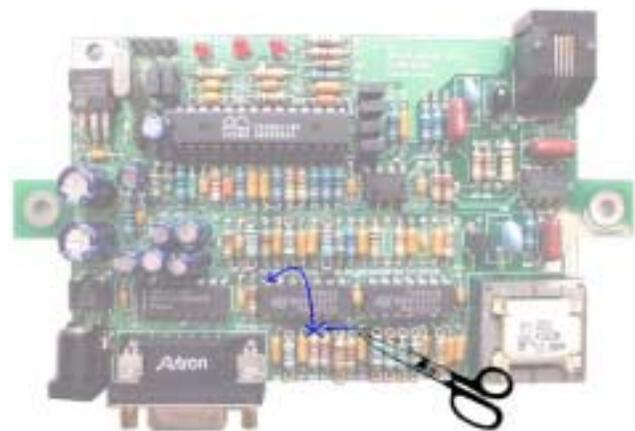
**Figure 6-1. DTMF HW Modification for the Modem Board**
