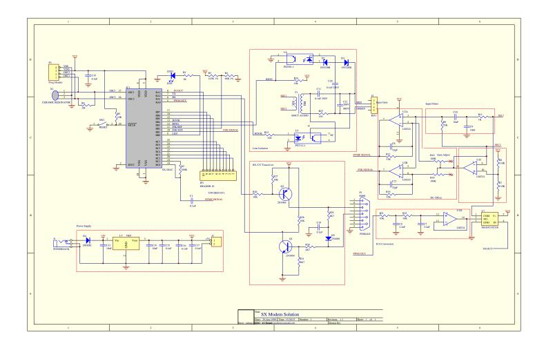
This schematic shows the latest revision of the hardware. Since the design of this board, we have found that much of the hardware is unnecessary, such as the potentiometers, the analog switch, the comparator reference resistors, and, quite possibly, the op-amp. Keep in touch with <u>www.scenix.com</u> for any updates we make available.
