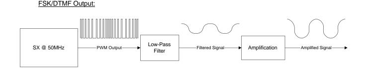
To convert the internal digital values inside the SX back into real-world analogue signals, a Digital-to-Analogue converter (D/A) is required. The SX modem uses a single 8-bit PWM virtual peripheral to accomplish the conversion. A PWM register is loaded with a value from 0 to 255, and this value represents the duty cycle of the PWM output. For DTMF generation, the PWM register is loaded with the sum of the amplitudes of each of the sine waves representing the digit.
